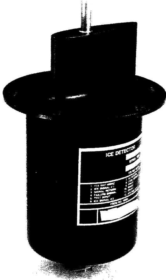
FIGURE 2 - SELF-CONTAINED B-747/B-767 ICE DETECTOR USING MAGNETOSTRICTIVE VIBRATORY PRINCIPLE
