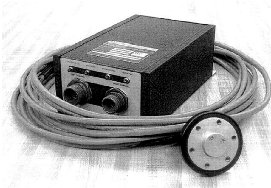
FIGURE 5 - FLUSH-MOUNTED ICE DETECTOR USING A MAGNETOSTRICTIVE VIBRATED DIAPHRAGM
