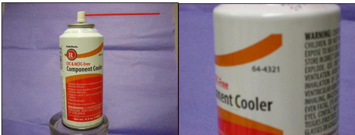
Figure 8 a, b -- Commercial component cooler spray freezes moisture out of the ambient air, simulates detectable ice.
