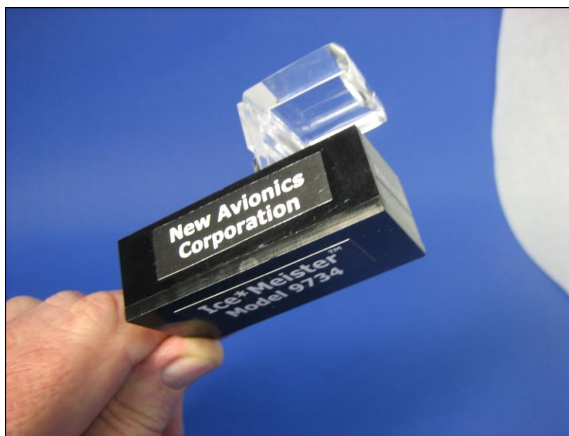
Figure 1 -- Model 9734-REFR demand defrost controller for commercial walk-in refrigerators and reach-in refrigerated display cases in supermarkets, restaurants, convenience stores.
