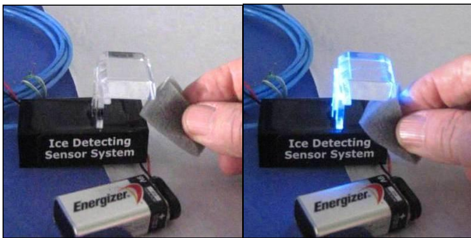
Figure 6-- Desktop FROST test with supplied 9-volt battery and opaque charcoal test foam.
