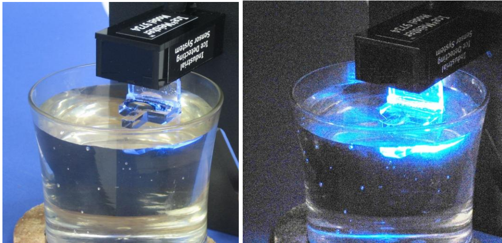
Figure 8-- CLEAR ICE test with 9-volt battery and clear glass tumbler of clean tap water.
