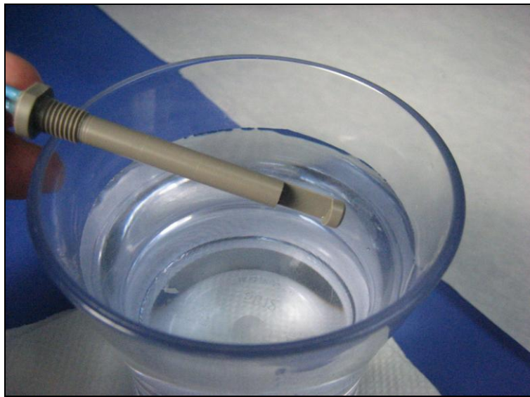
Figure 10 – Ordinary clean tap water simulates clear ice.
