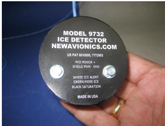
Figure 5 -- 9732 installs with (2) #6-32 screws through wing and directly through the epoxy-filled body of the unit. The steel probe's 5/16-24 thread provides the third attachment screw.
