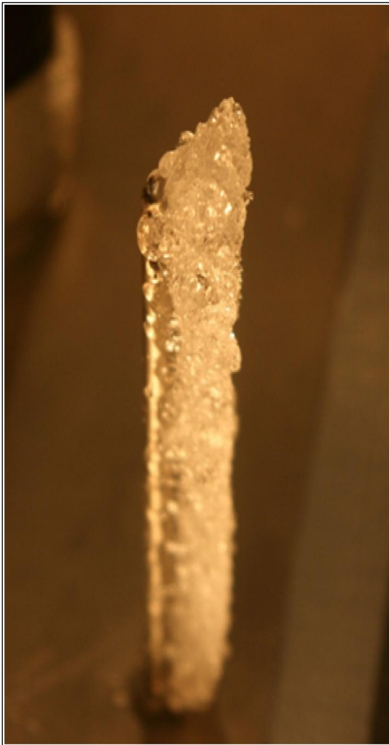
Figure 15 -- ice formation on sensor probe is by nature rough, imprecise, "fuzzy".
