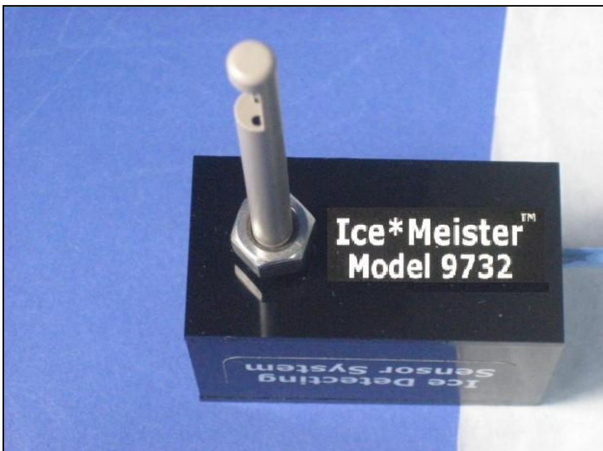
Figure 1 — Model 9732-PLASTIC aviation ice detector is a commercial, off-the-shelf, in-flight ice sensor that monitors the optical characteristics of whatever substance is in contact with the optical surfaces of the probe, either air (NO ICE) or water ice (ICE ALERT). Ambient wind blows standing water away, but ICE sticks. Made of nonconductive *PLASTIC, probe is electromagnetically compatible with its host aircraft's radio environment.
