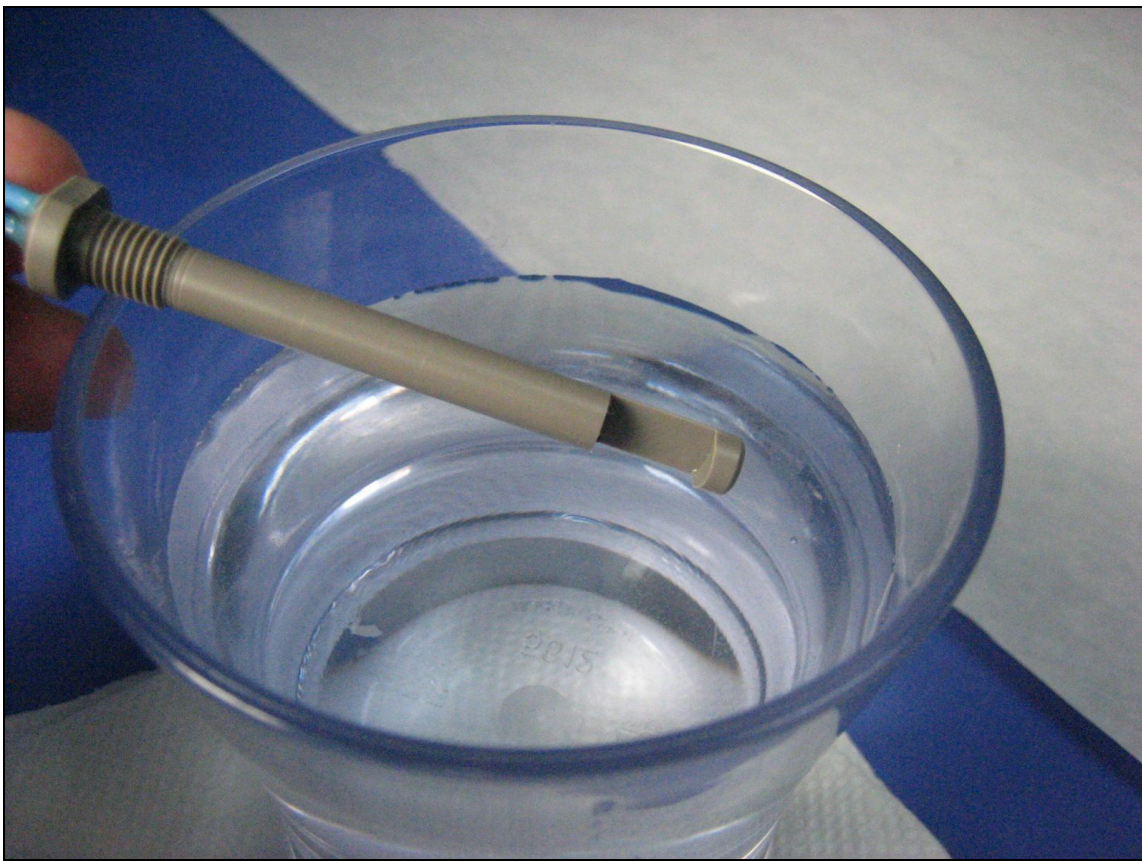
Figure 10 – Ordinary clean tap water simulates clear ice .
