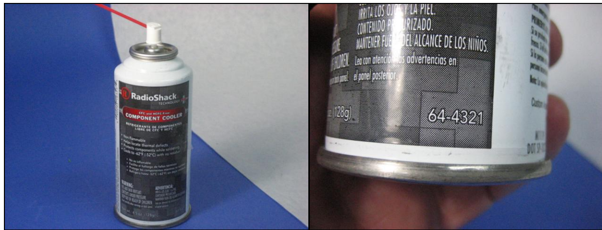
Figure 9 a,b -- Radio Shack component cooler. Be certain to use ONLY tetrafluoroethane component cooler to avoid damage to the acrylic optical components in the air gap.
