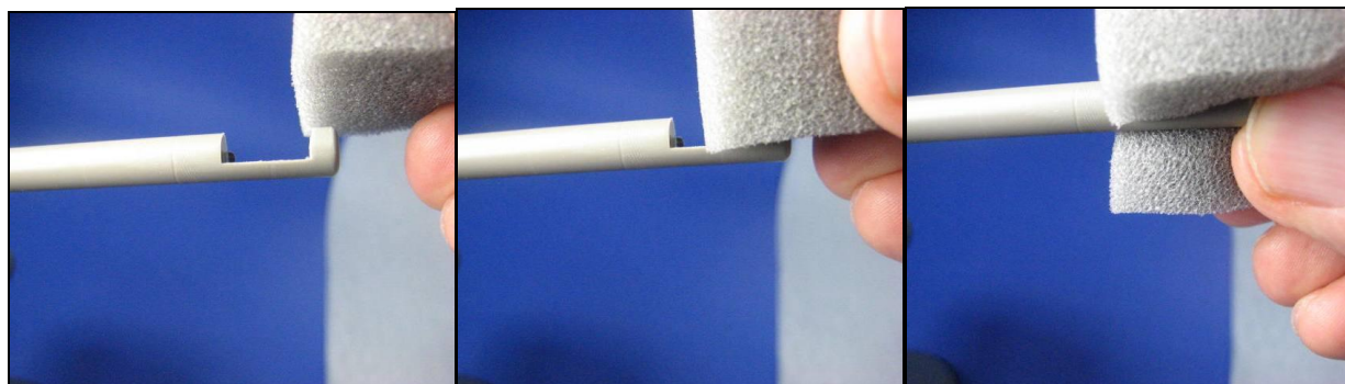
Figure 11 a, b, c -- Field test for progressive rime ice by blocking the optical air gap with a piece of readily available charcoal packing foam -- soft, dry, resilient, opaque, non-reflective.
