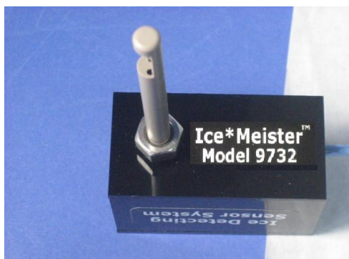
Figure 1 — Optical aviation ice sensor is a commercial, off-the-shelf, in-flight ice sensor that monitors the optical characteristics of whatever substance is in contact with the optical surfaces of the probe, either air (NO ICE) or water ice (ICE ALERT). Ambient wind blows standing water away, but ICE sticks. Made of nonconductive delrin and acrylic plastics, probe is electromagnetically compatible with its host aircraft radio environment, and can be installed in close proximity to radio antennas.
