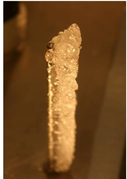
Figure 4 -- Saturation ice on an Ice*Meister™ Model 9732 ice detecting sensor for aircraft
