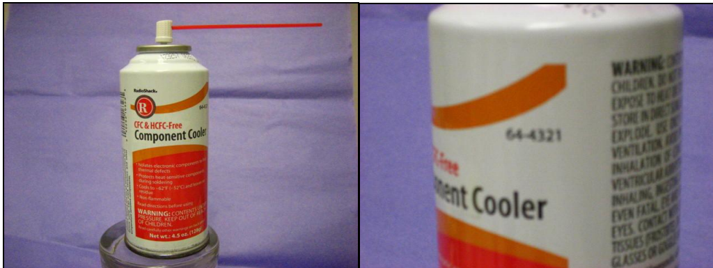
Figure 11 -- Commercial component cooler spray simulates detectable FROST on the evaporator coil.
