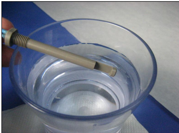
Figure 10 – Ordinary clean tap water simulates clear ice.
