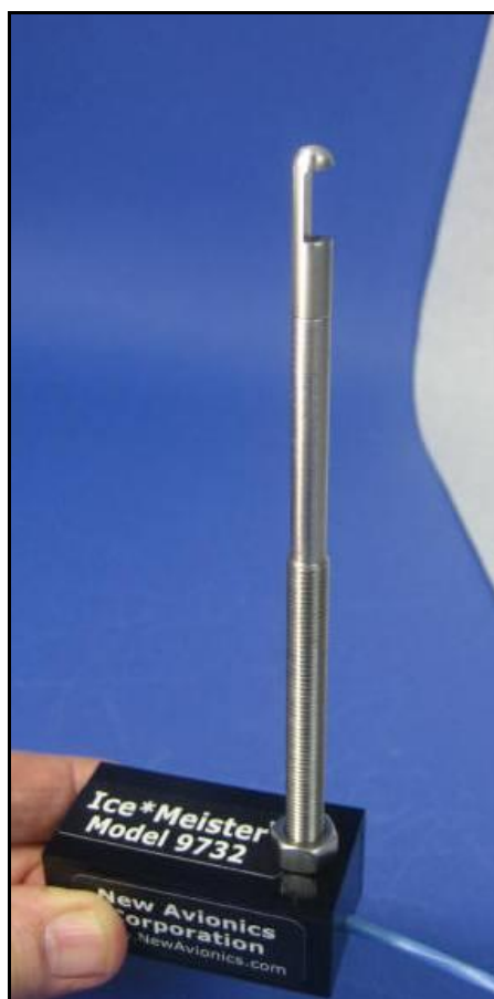
Figure 1 — Model 9732-STEEL aviation ice detector is a commercial, off-the-shelf, in-flight ice sensor that monitors the optical characteristics of whatever substance is in contact with the probe, either air (NO ICE) or water ice (ICE ALERT). Reports rate-of-ice-accumulation in three stages. Acrylic housing is size and shape of a hockey puck. * Probe is type 316-L marine grade stainless steel for subsonic flight. See fig 2.
