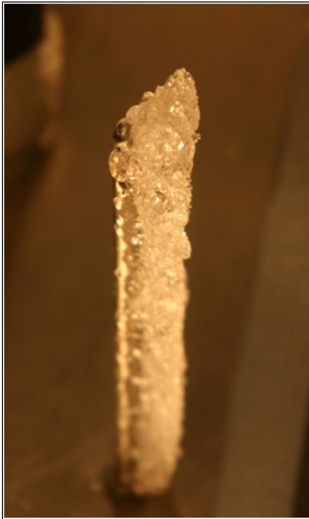
Figure 12-- ice formation on sensor probe is by nature rough, imprecise, "fuzzy".
