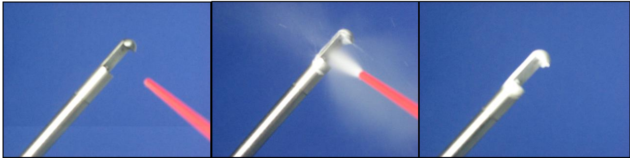
Figure 8 a,b,c – Primary test mode simulates rime ice by using cold spray.
